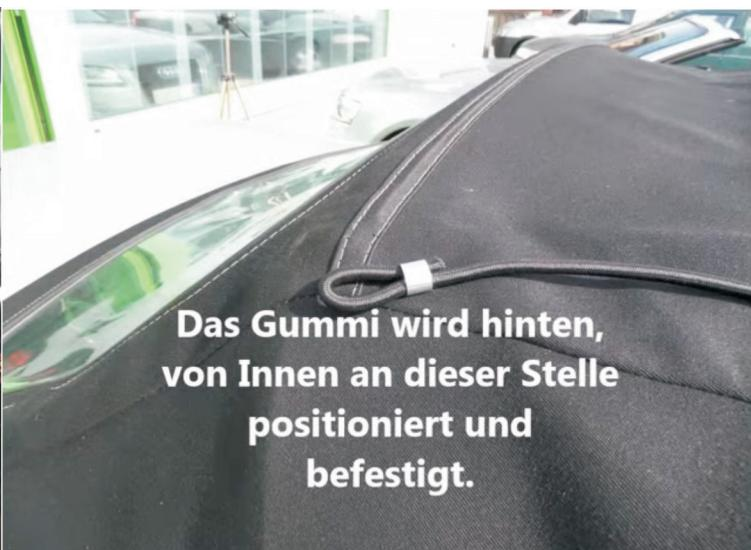
The expander has to be placed on the inside like shown on the photo
