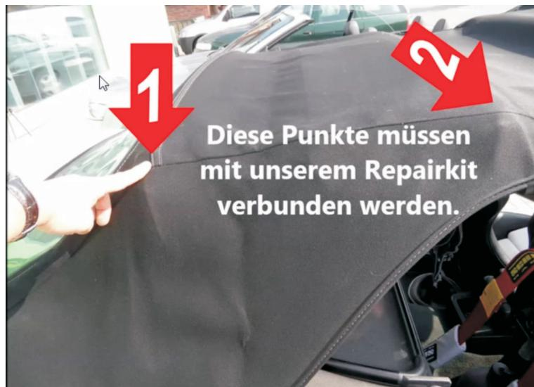
Pos.1 and 2 have to be connected through our repair-kit
