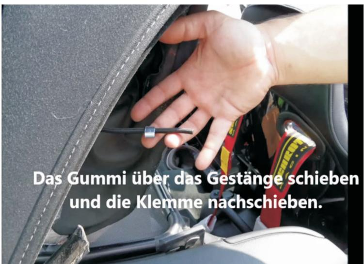
Thread the expander over the struts and push on the crimp
